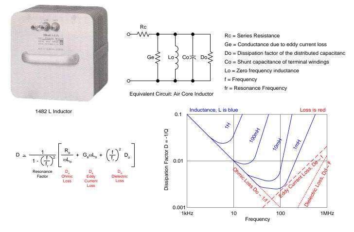
Figure 5: 1482 Inductance Standard Loss Curve
